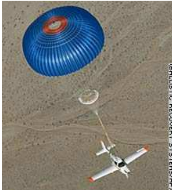
Figure 1: Ballistic Recovery Systems and NASA are designing a parachute for small planes.
